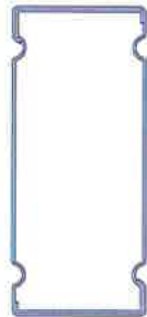
150 x 65 x 1.2mm G550 Roll Formed Box Beam
